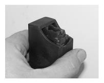
② Place bullet in magazine and push bullet fully rearw the plunger of the loader.
