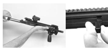
(5) Place MAX-11mk2/22 bolt assembly on top of barrel insert/ejector plate.
