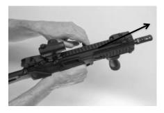
(3) Remove front retaining pin and remove upper receiver from lower receiver.
