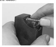
(6) Release loader and lightly push bullet until it contacts the rim of the bullet previously loaded.
