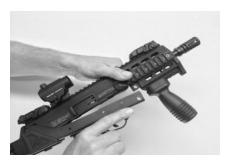
(9) Insert upper receiver retaining pin.
