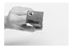
(6) Install assembly inside upper receiver insuring barrel insert is placed inside barrel. Slide assembly forward until cocking knob slot lines up with rear of slot in upper receiver. Install cocking knob.
