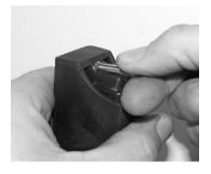
(3) Release loader and lightly push the bullet until it seats against back wall of magazine.
