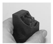
(5) Place bullet in magazine and push bullet fully rearward until it seats against the plunger of the loader.
