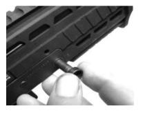
(1) Cycle the bolt back and forth to insure there is no binding and that it seats fully closed.
