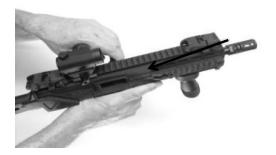
② While holding cocking knob, pull trigger and ease bolt forward into closed position.
